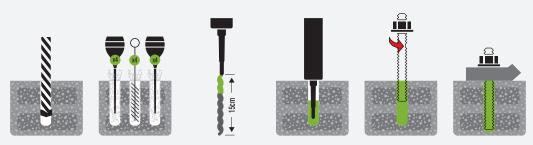
For new cartridges dispense a bead of adhesive until even and consistent colour is present to ensure correct mix of adhesive.
